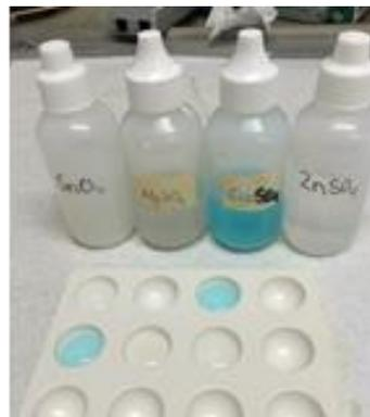
2. Be sure to know which metal strip is which. Writing the names down on a paper and placing the metals back where they belong is a good method to not mix them up. If any of the pieces of metal have a coating or discoloration on them, light sanding can clean them up.
