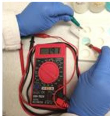
7. Once the voltage of that metal combination has been recorded, remove the strips from the wells and the alligator clips and place them back on the paper with their names. Remove the salt bridge from the wells and discard it. **Never reuse a salt bridge or your metal solutions and all future readings will be compromised.**
