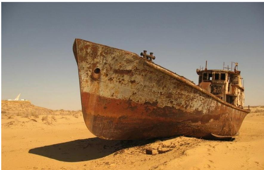
Figure 1. The formation of rust on an old ship is an electrochemical process that forms iron oxide.
